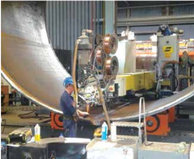
Figure 4. The formed plates are welded together internally and externally by a longitudinal weld.
