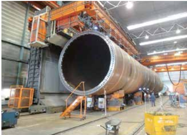
Figure 11-12. Sif manufactures XL monopiles from thermomechanically rolled steels from Dillinger in thicknesses of up to 140 millimeters.
