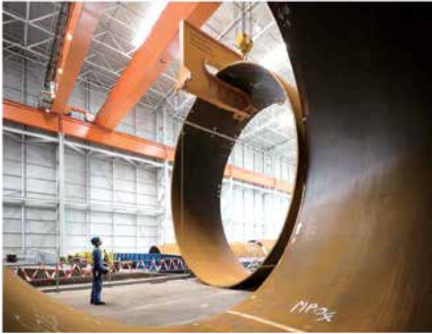
Figure 7. Huge crane systems transport the shell sections to the welding area.
