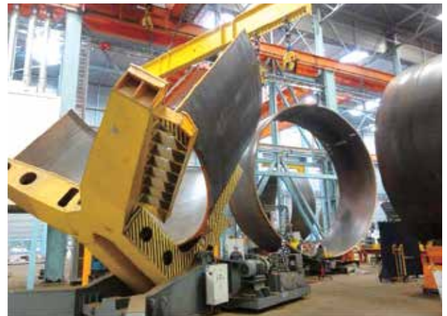
Figure 3. Rolling machines form the Dillinger plates into half-shells.
