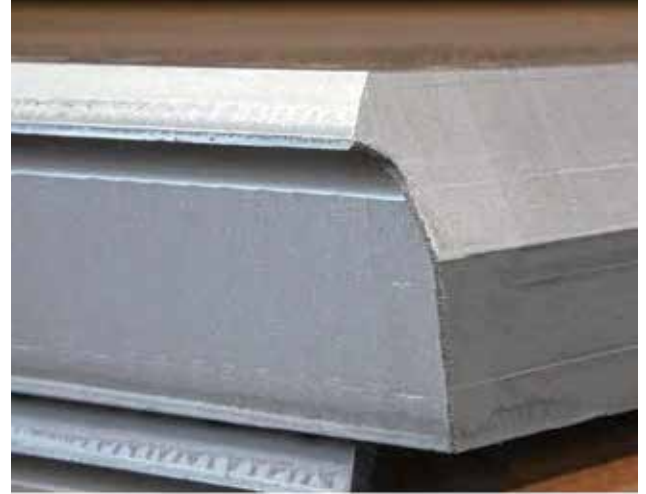
Figure 1-2. Dillinger supplies Sif with heavy plates weighing up to 32 tons and with thicknesses of up to 500 millimeters, some with milled edges already attached.
