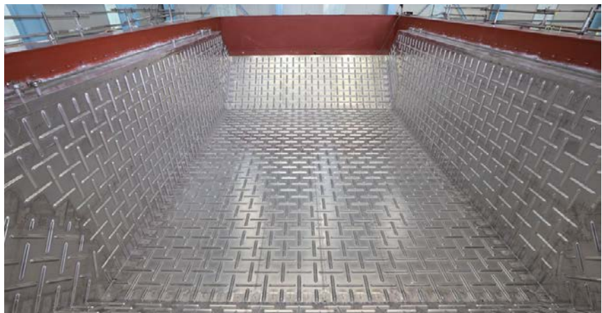
Life-size model of SOLIDUS, a LNG cargo containment system developed by DSME
