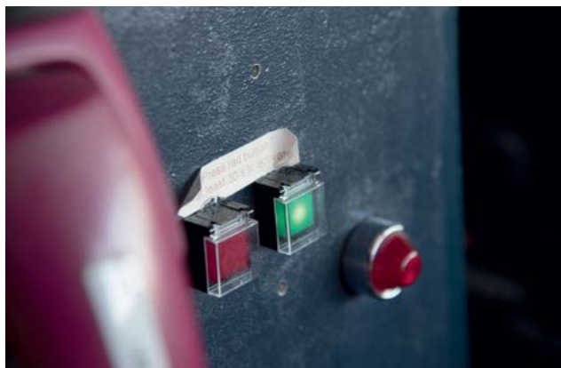
Figure 4. Inconspicuous placement, but a serious outcome: if both buttons are pressed in case of a pirate attack, a comprehensive crisis management program will run in the background.
