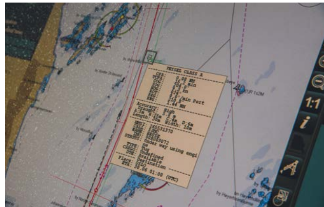
Figure 5. The AIS provides information about key data from other ships on the route.
