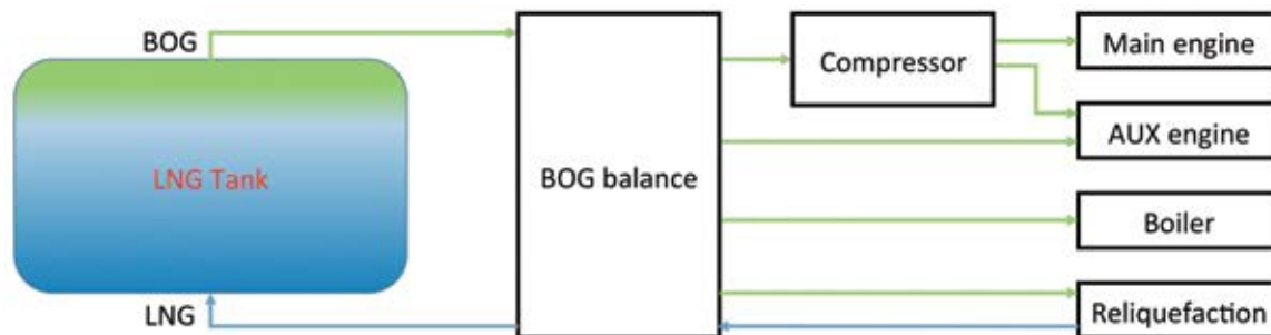
Figure 1. Simplified system layout for BOG handling, when using two-stroke main engines and four-stroke auxiliary engines. Ideally consumption should match BOR, resulting in a BOG balance of zero.
