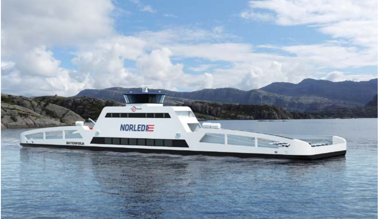
The ZeroCat 120 battery-powered ferry will have space for 120 cars and up to 360 passengers.
