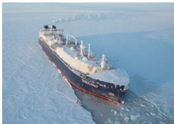
The world's first icebreaking LNG carrier built by DSME is cutting through the ice
