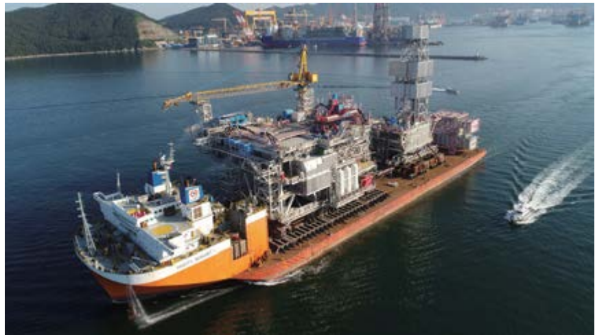
A fixed offshore plant built by DSME set sail in a barge for the North Sea continental shelf in the U.K. for installation.
