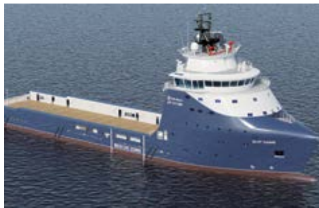
The UT 771 WP complements other PSV designs and can carry a range of cargoes in a safe and efficient way. It has a deadweight of 4,200dwt.
