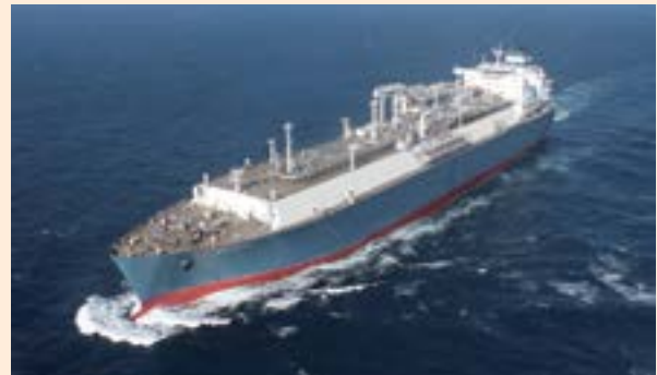
The world's first newbuilding 170,000 cbm LNG-FSRU that HHI built for Hoegh in 2014.
