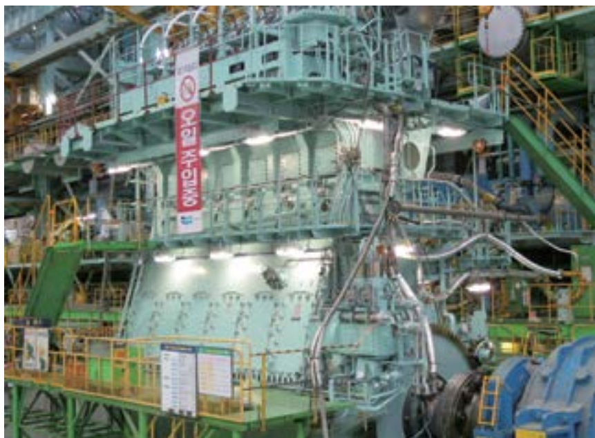
The X62DF dual-fuel engines with X-DF low-pressure gas injection technology designed by WinGD will power four ice class 1A, 114,000 DWT Aframax tankers of SCF Group.
