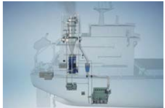
Example of a DeSOx Scrubber
