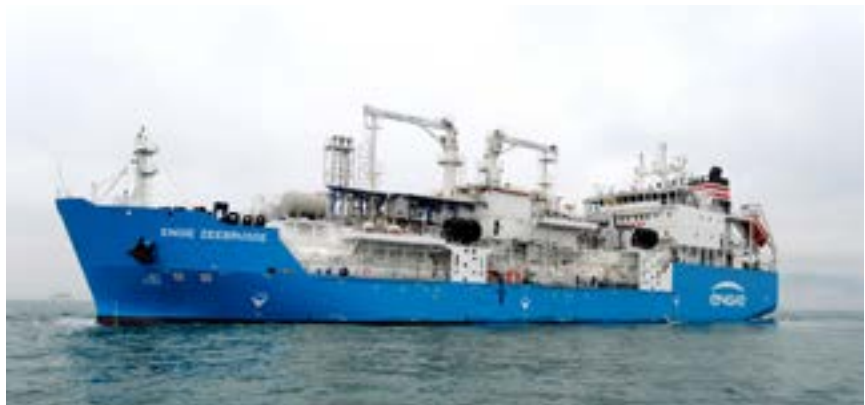
5,100m 3 LNG bunkering vessel "ENGIE ZEEBRUGGE" built by HHIC
