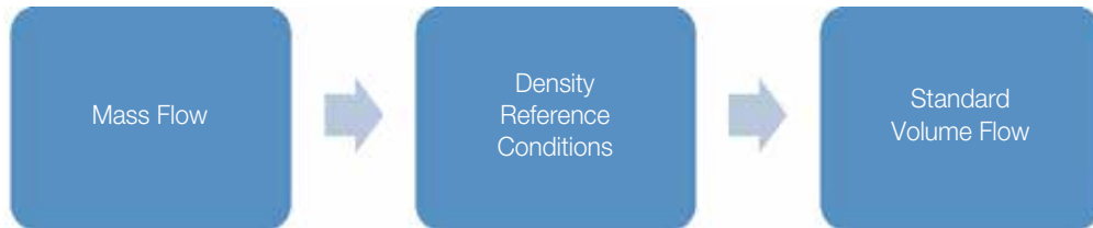
Figure 7. Mass flowmeters require the knowledge of the density of the gas at reference conditions in order to output standard or normal volume flow. For constant composition gases, this will be a constant number. For changing composition gases, this number will vary and additional equipment (like a gas chromatograph or specific gravity meter) may be required.
