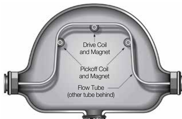
Figure 4. A typical curved tube Coriolis flowmeter has two parallel tubes that are vibrated at their natural frequency. All flow is split and flows through the bent tubes.
