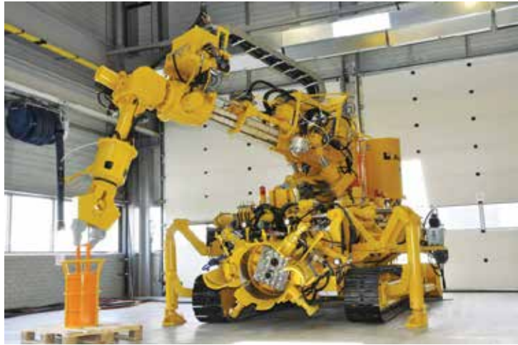
The Subsea Crawler from Aker Wirth with modified hydraulics by Rexroth.
