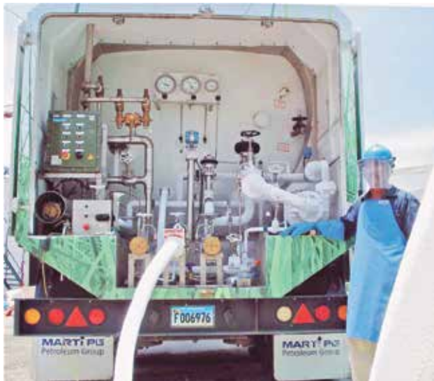
Figure 3. Unloading an LNG truck can be a one man operation. The LNG tank in the truck is at a higher pressure than the recipient allowing LNG to flow from it without the need of any pumps. A clever, simple system.
