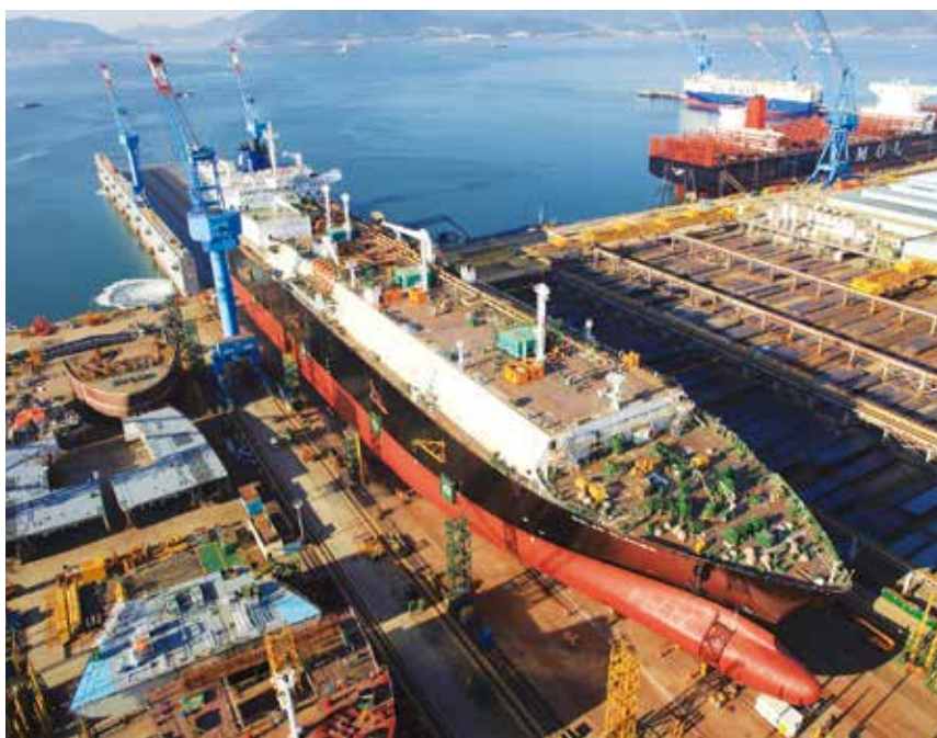
Aerial view of launching LNG Carrier built on-ground
