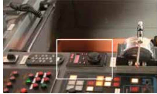
The FLIR M-Series thermal imaging camera's control unit is seamlessly incorporated in the bridge.
