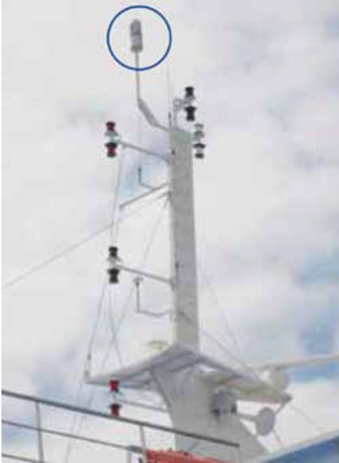
The FLIR M-Series thermal imaging camera is mounted on a pole for a better situational awareness and a better range performance.
