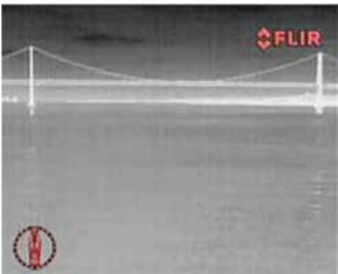
The FLIR M-Series thermal imaging camera enables the captain of the Lisbonense to avoid collisions even if light fog, smoke or darkness impedes vision.
