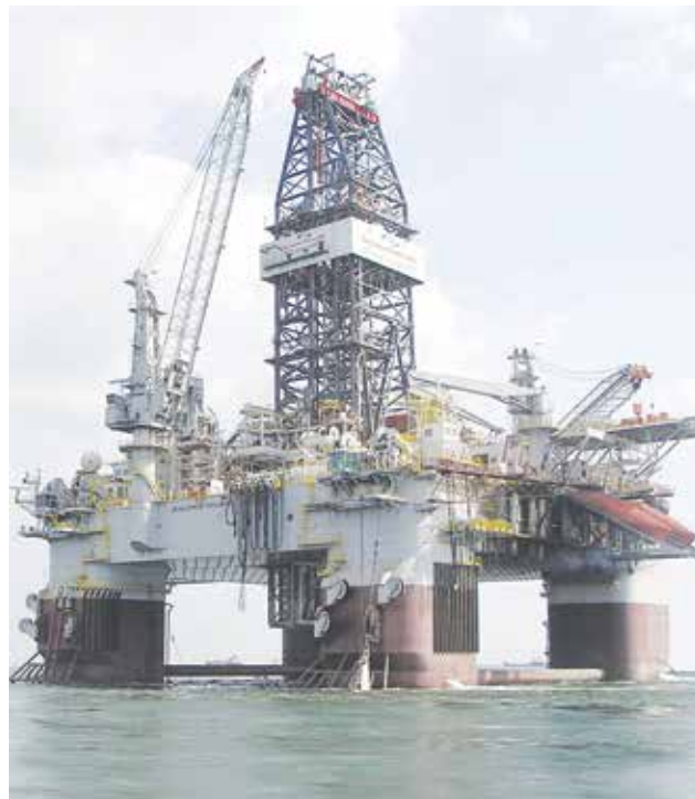
Figure 6. Development Driller I (shown above) and Development Driller II from Transocean (originally built for Global Santa Fe) are both equipped with Azipod® CZ thruster systems.
