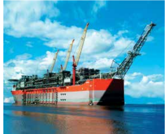
Large-scale FPSO with a storage capacity of 2 million barrels, built by SHI
