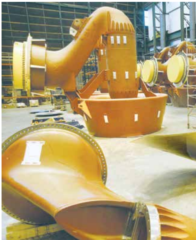
Figure 2. Azipod® CZ presents a significant advancement in thruster technology for drilling vessels with station keeping capabilities.
