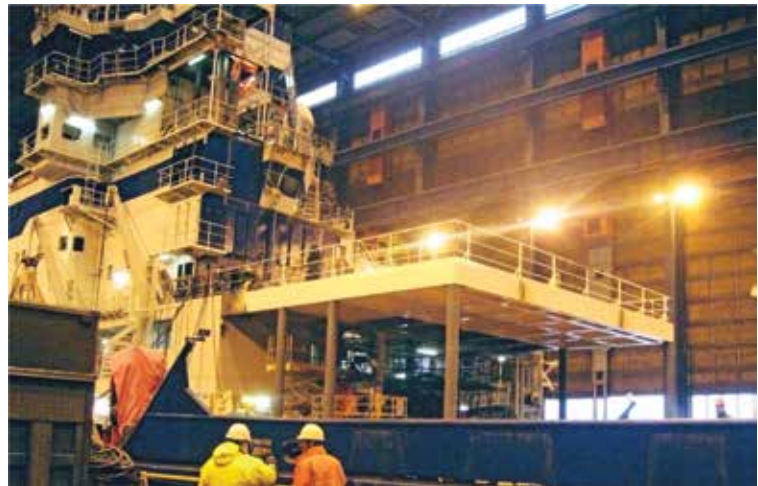
Figure 4. The deck extension installed.
