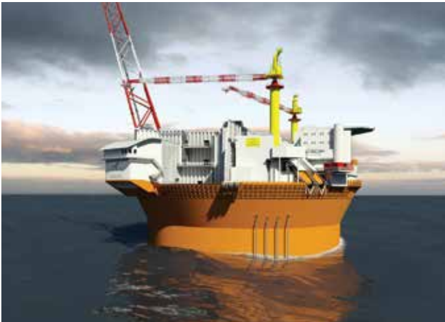
Bird's eye view of the Goliath FPSO of Hyundai Heavy Industries(HHI). Goliath FPSO has a cylindrical design to withstand the freezing cold weather and strong waves.
