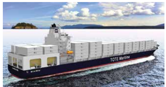
Figure 4. Model of TOTE's containership equipped with ME-GI, the world's first LNG-powered vessel
