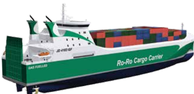
JD 4103 GF ro-ro cargo carrier - 9,000dwt/1,750lm
