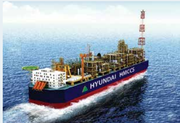
Bird's eye view of LNG FPSO fitted with membrane type LNG cargo containment system
