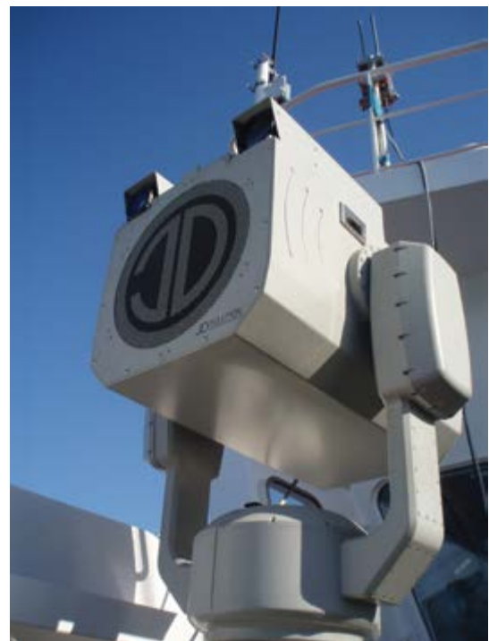
The sound cannon installed in the oil tanker currently being built.
