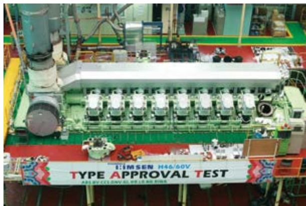
HHI's 35,300-horsepower HiMSEN Engine(model name: H46/60V), which received the type approval from 9 classification societies.
