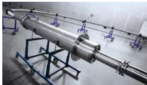
This prototype of a superconductive cable system for Essen city centre was put through its paces in the high-voltage laboratory in Nexans’ Hanover plant.
