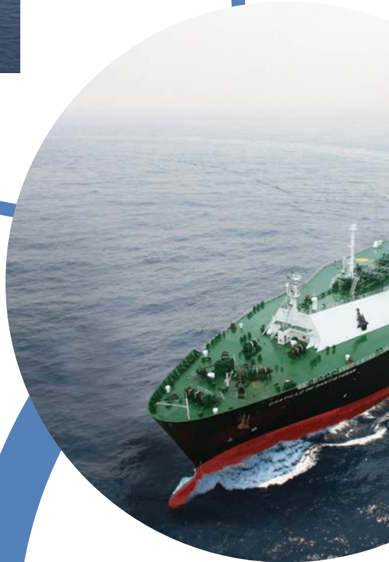
173,600CBM ultra large LNG carrier built by STX
