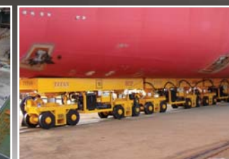
RTP (Transfer System) CAPACITY: 100TON ~ 600TON FOR COMBINATIONS OF UP TO 90,000TON
