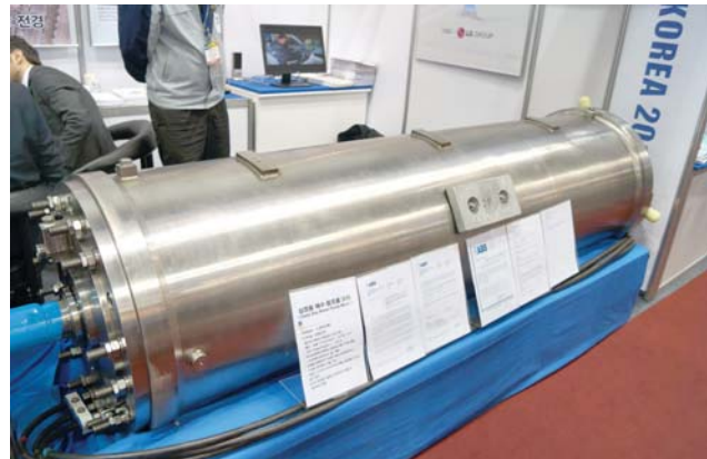
Deep sea water pump motor
