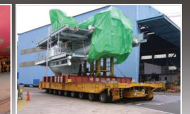
SSC (Ship Section Carrier) CAPACITY: 50TON ~ OVER. 1,000TON FOR COMBINATIONS OF UP TO 10,000TON
