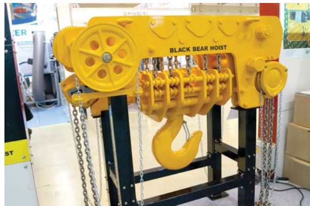
Low Headroom Hoist of Black Bear Hoist
