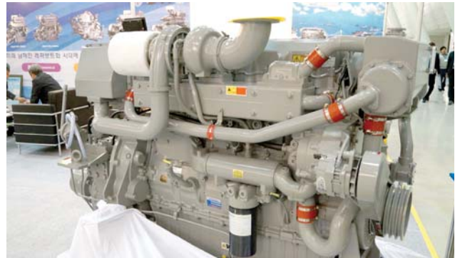
Diesel engine for small-to-medium sized ships - DD6CC 500PS/550PS 2000RPM
