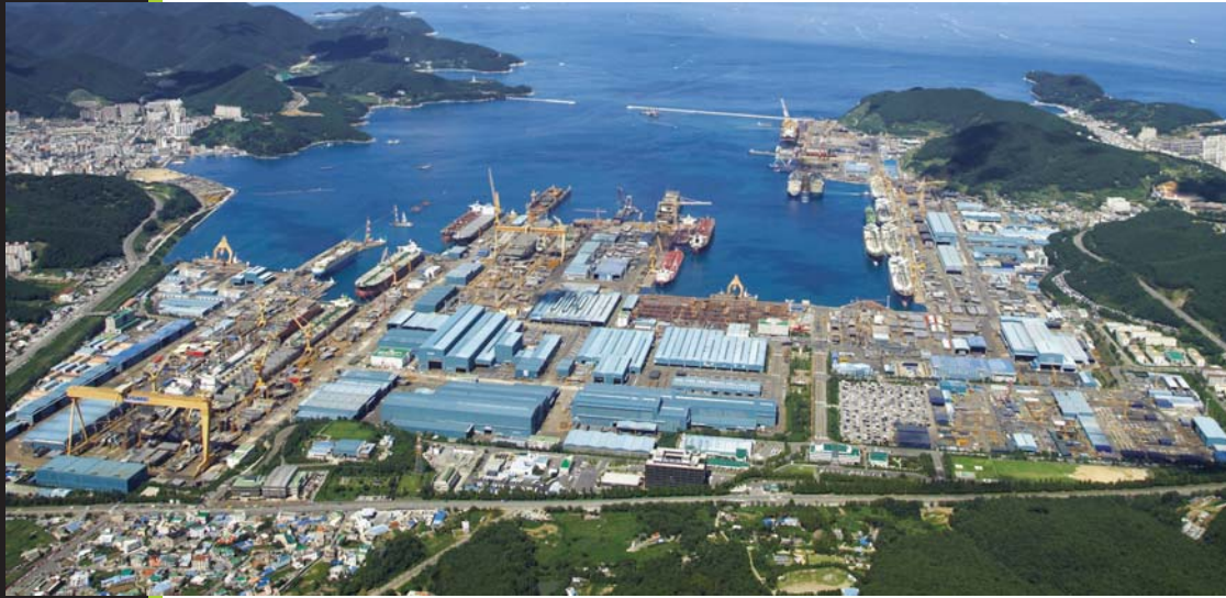
Daewoo Shipbuilding & Marine Engineering (DSME) uses factory area of 351,000m 2 among total 4million m 2 yards, 4,988m of outfitting quay, 11.3m of quay water level, 0.2m of surrounding average wave height, 17.5°C of average temperature, where is 40 commercial ships, 100,000tons of land and marine plants, submarine, war ship and various special ships are built in the facility.
