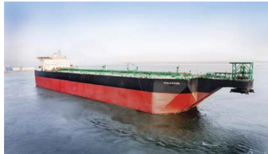
FSO with a storage capacity of 2.2 million barrels, built by STX.
