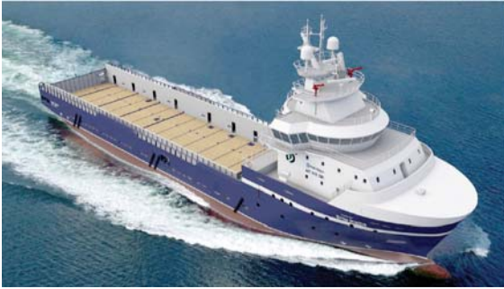
This vessel is an OSV which Island Offshore ordered to STX OSV. This vessel measures 84.3m in length, 17m in width with a deadweight tonnage (DWT) of 3800, and features the UT 717 CD design of Rolls-Royce.
