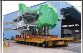
SSC (Ship Section Carrier) CAPACITY: 50TON ~ OVER. 1,000TON FOR COMBINATIONS OF UP TO 10,000TON
