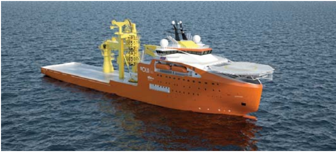
This vessel, built by STX OSV, was designed to carry out the installation of SURF (Subsea, Umbilicals, Risers, Flowlines) that transports the oil and gas, produced from under the sea bed, to the offshore storage facility.
