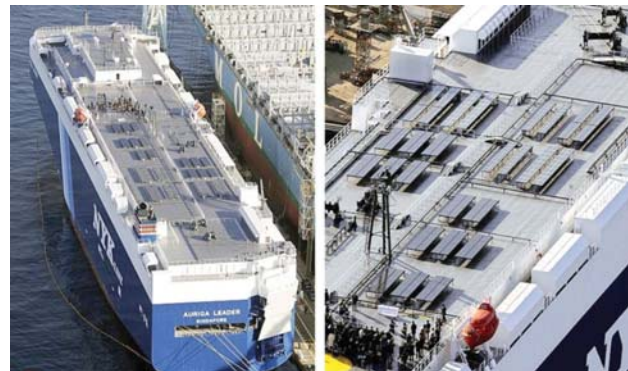
Figure 11. NYK Line equipped with solar photovoltaic power generation system.
