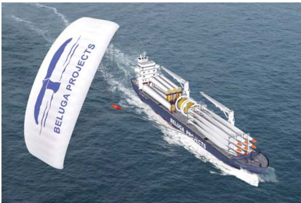
Figure 12. Ship equipped with the kite of Skysails.
