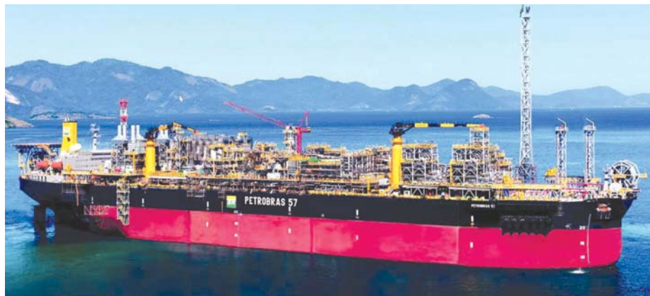
The upgrading and pre-conversion of the 255,272 dwt tanker, Accord, into the P-57 was completed at Keppel Shipyard in Singapore earlier in 2010. The engineering was done in Schiedam. SBM delivered the FPSO to the owner, Petrobras Netherlands. The FPSO operates in the Jubarte Campos Basin which is 70km offshore the state of Espírito Santo, Brazil. Photograph courtesy of Mercator Media.
