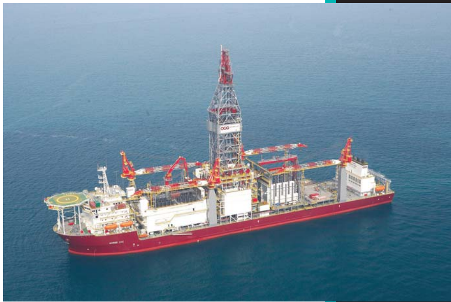
'Norbe VIII', a drillsip built with the independent technology (DSME-10000 type) of DSME, can operate in water depth of up to 10,000 feet. It is equipped with the cutting-edge position control system and drill up to 12km below the sea surface, drilling deeper than the height of Mt. Everest (8848m).
