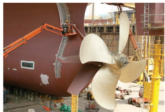
Figure 5. Pre-Swirl Stator by Daewoo Shipbuilding & Marine Engineering
