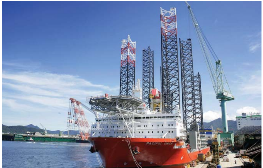
'PACIFIC ORCA', the world's largest Windfarm Installation Vessel
