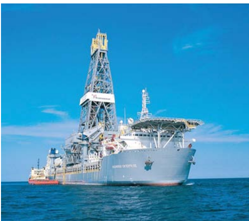
The Discoverer Enterprise of Transocean is the first ultra-deepwater drillship with dual activity drilling technology.
