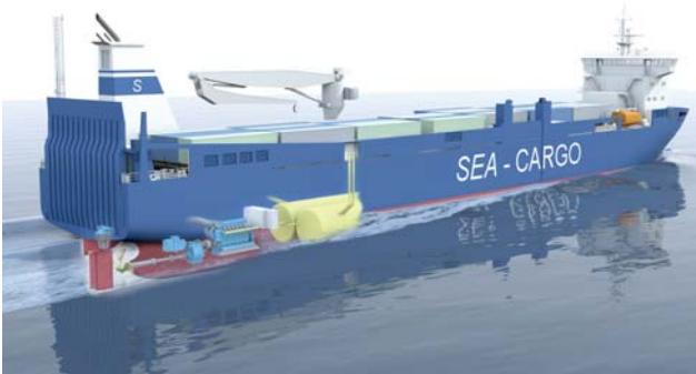
The propulsion system for two new Sea Cargo vessels uses a single Bergen V12 gas engine driving a PROMAS integrated propeller rudder system for maximum efficiency and low environmental impact.
