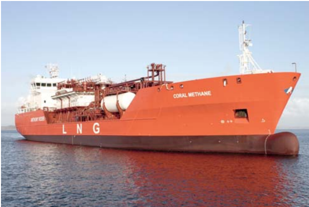
The innovative gas carrier Coral Methane has a Rolls-Royce supplied electric propulsion system and can use either twin Bergen gas or diesel engines depending on the cargo carried.
