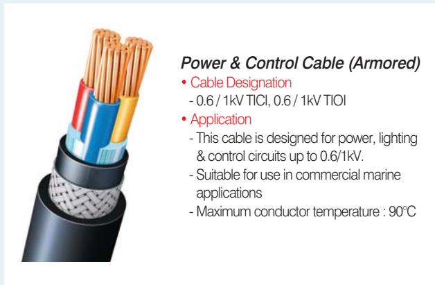
Figure 4. Halogen Free Shipboard Cables (XLPE Insulation / SHF1 Sheath Cables)
