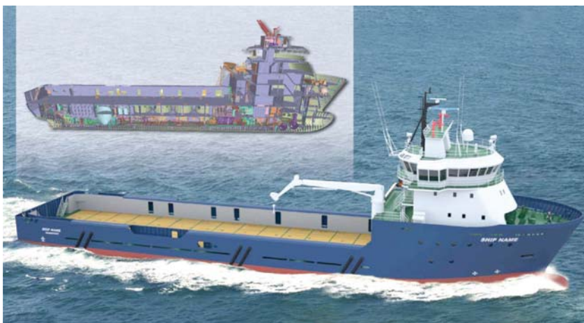
The UT 755 series has generated more than 180 vessels either currently in service or on order worldwide. Photograph courtesy of Rolls-Royce. AVEVA Marine model of a platform supply vessel (PSV) of the UT 755 CD design.
