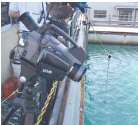
These FLIR thermal imaging cameras are pointed at oil spills in the OHMSETT tank at different angles.
