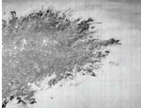
The oil spill shows up clearly on this thermal image.
