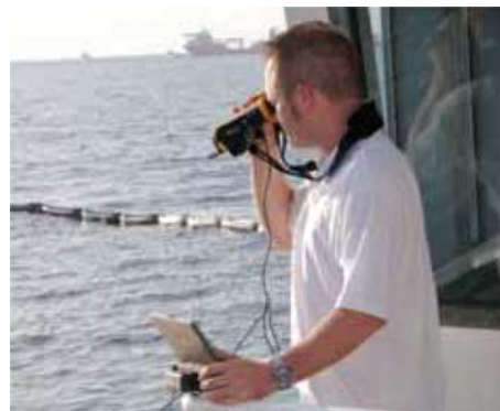
An oil recovery operator uses a FLIR HM-Series handheld thermal imaging camera to direct the positioning of oil recovery booms.
