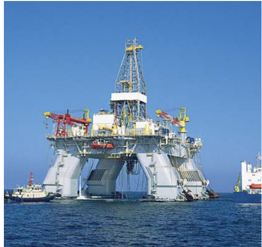
Deepwater Nautilus. Hyundai Heavy built this semi-submersible drilling rig for Transocean in 1999.
