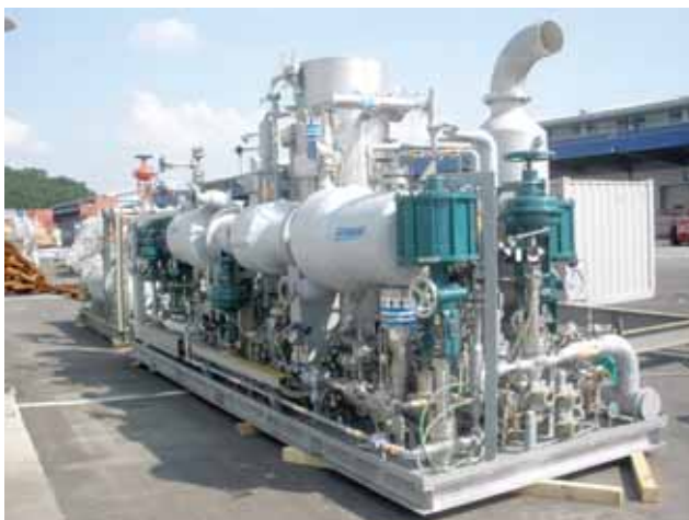
Figure 9. High pressure fuel gas supply system (HP-FGS) of DSME.
