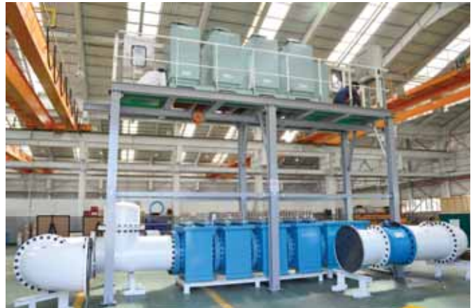
AquaStar™ BWMS H-650(3000m 3 /hr) installation (Daisy, Polaris shipping)
