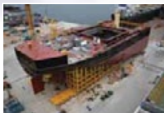
MTP (Module Transporter) CAPACITY: 60TON ~ 1,000TON FOR COMBINATIONS OF UP TO OVER. 20,000TON
