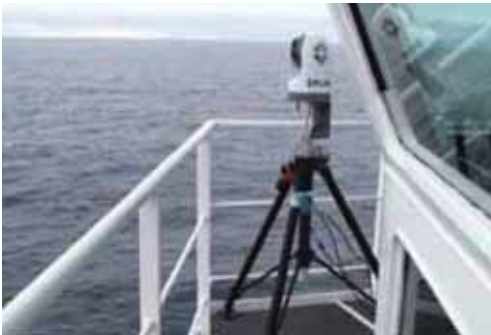
For the test two models of the M-Series were mounted on a tripod next to the bridge of an ice strengthened vessel that traverses the Arctic waters of Greenland.
