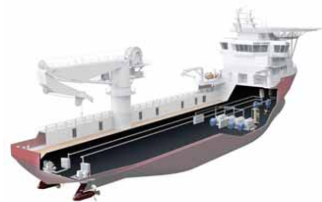
Figure 1: Platform Supply Vessel with Onboard DC Grid
