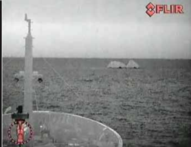
The searchlight only illuminates objects in the narrow path of its lightbeam. A thermal imaging camera presents a much wider view, resulting in better situational awareness.
