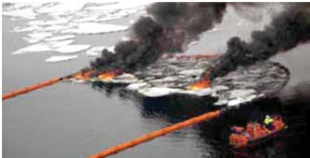
Oil spill exercise: burning of oil in water is an option for combating oil spills in arctic waters. (source: SINTEF)
