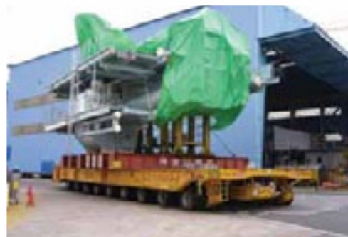
SSC (Ship Section Carrier) CAPACITY: 50TON ~ OVER. 1,000TON FOR COMBINATIONS OF UP TO 10,000TON
