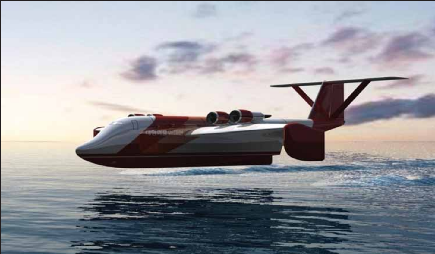
Bird's eye view of large wing-in-ground craft with a carrying capacity of 350 passengers
