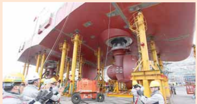
The azimuth thruster is being installed on land at the onshore dock of DSME's Okpo shipyard.
