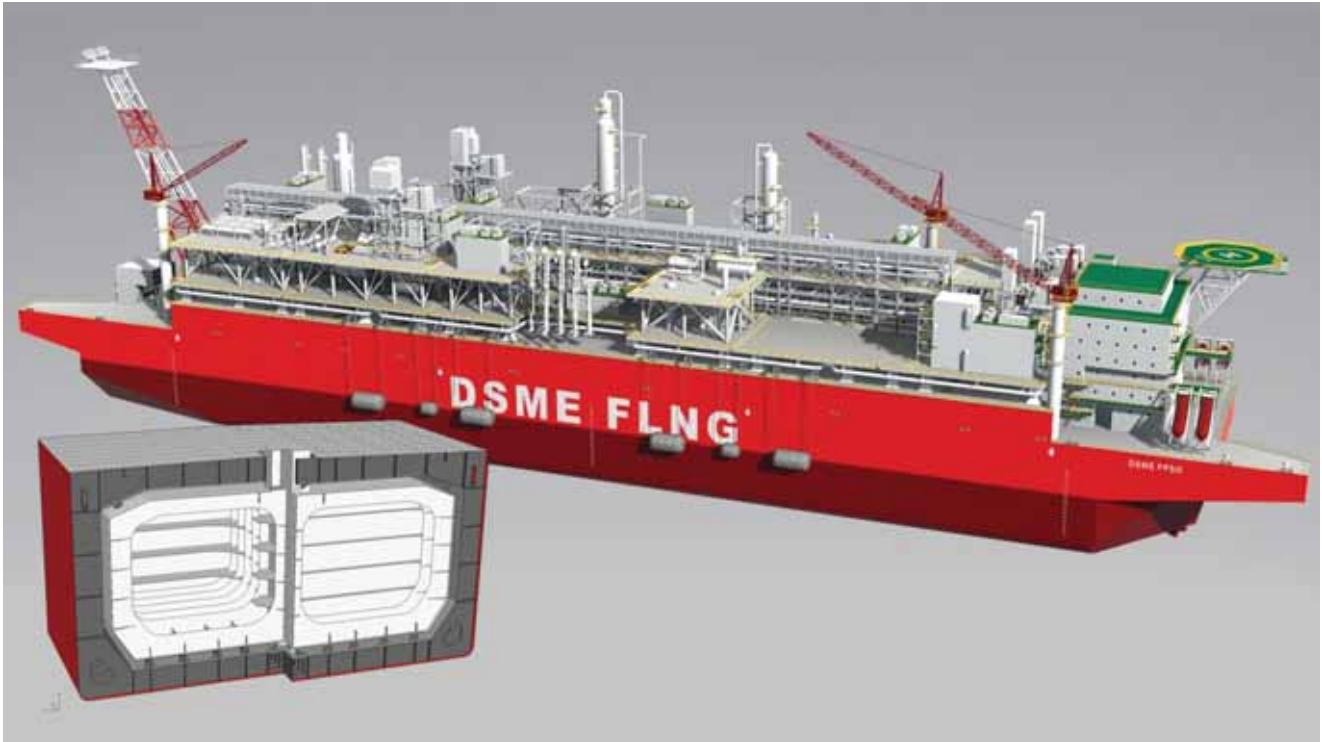
Schematic diagram of 'ACT-IB (below)', the independent type LNG storage cargo containment system developed by DSME, and LNG-FPSO (above) fitted with it.
