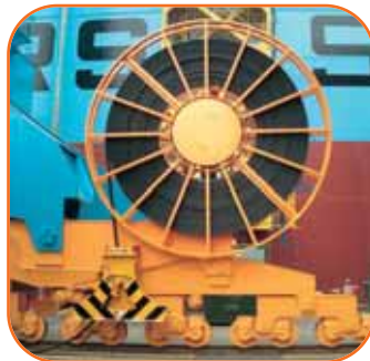
☞ Cable reel installed in Hanjin Heavy Industries & Construction
