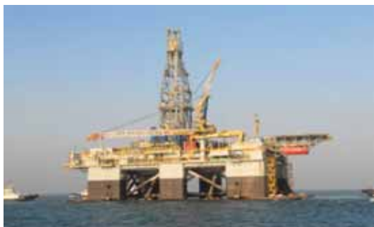
Noble NDB, a semi-submersible deepwater drilling platform Source: Website of CSIC
