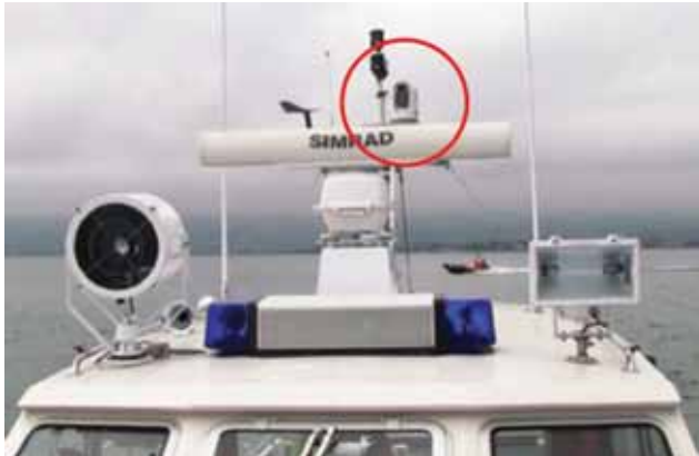
The FLIR M-Series thermal imaging camera is mounted on top of the bridge to provide a good range performance.
