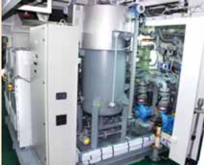
'HiBallast', a ballast water treatment system, for which HHI won type approval recently
