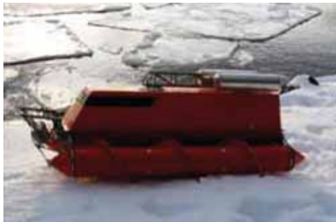
Evacuation vessels advances in water and on ice using Archimedes' screw for propulsion. Photo: Sveinung Løset
