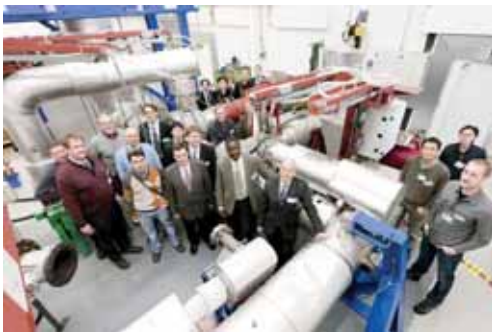
Power2 two stage turbocharging on the test bed at the ABB Turbocharging technical centre.
