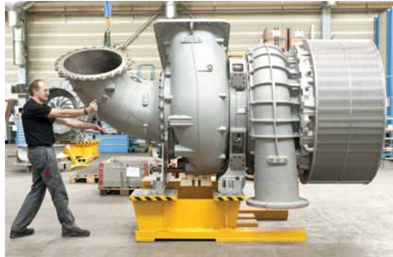
ABB Turbocharging's A190-L turbocharger for 2-stroke low speed engines.
