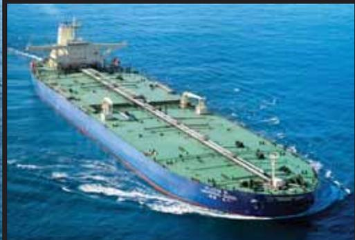
309,000DWT VLCC built by HHI
