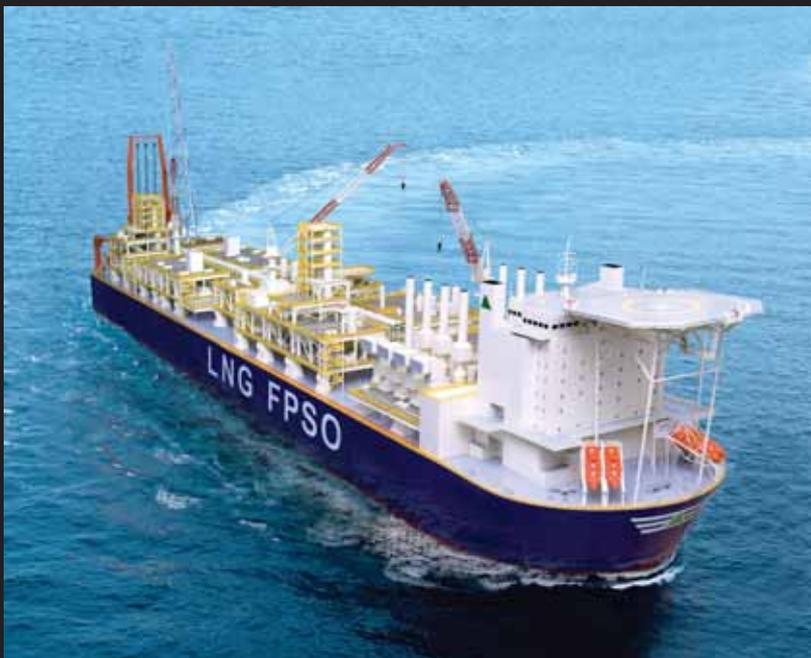
LNG-FPSO (LNG-Floating Production Storage-Offloading) of HHI
