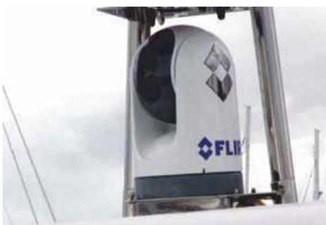
The FLIR M-625L on the Navetta 26 contains both a thermal imaging camera and a daylight/lowlight camera.
