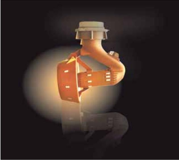
Azipod CZ electric podded thruster unit
