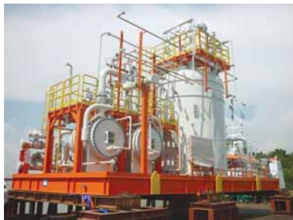
TGT-produced water treatment: Hydrocyclones and Induced Gas Flotation /Bumi Armada)
