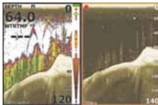
**-DownScan Overlay Illustrated:** These screen shots of a sunken bridge support in a Montana lake clearly displays the difference DownScan Overlay can make. Compare the lower right sonar windows of each. Without overlay (up), Broadband Sounder structure showing is excellent, but not well-defined. By adding DownScan Overlay (down) the structure - and fish - are clearly displayed.
