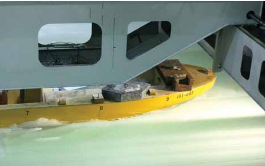
Final performance test of HHI's icebreaking commercial vessel model in an ice tank at the IOT in Canada
