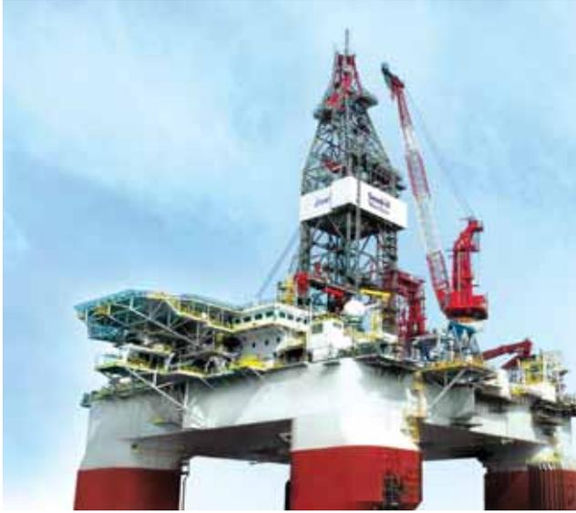
West Sirius was delivered to Seadrill in 2008 from Jurong Shipyards. This 6th generation semi-submersible drilling rig is equipped with Power Generation and Distribution systems, Thruster Drive systems and Drilling Drive Systems from ABB.
