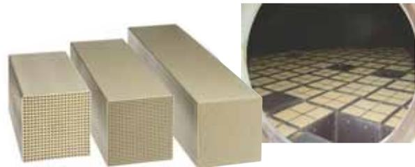
Shape of catalyst (left) and the installed appearance (right)
