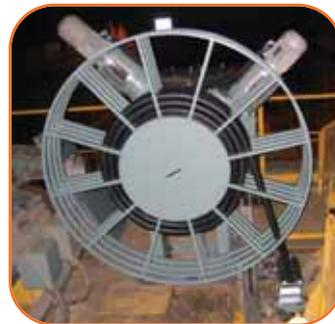
☞ Cable reel installed in Hyundai Hysco
