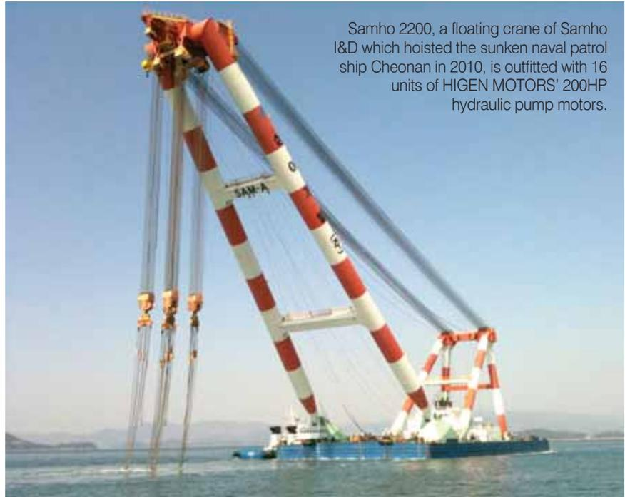
Samho 2200, a floating crane of Samho I&D which hoisted the sunken naval patrol ship Cheonan in 2010, is outfitted with 16 units of HIGEN MOTORS' 200HP hydraulic pump motors.
