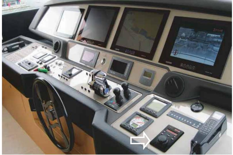
The thermal images are shown on a dedicated screen on the bridge. The joystick control-unit is aesthetically integrated.
