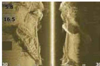
**-DownScan imaging:** The SIMRAD innovation of dedicated sounding focused vertically beneath user's vessel removes all guess-work in
