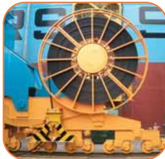
☞ Cable reel installed in Hanjin Heavy Industries & Construction
