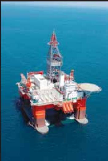
Semi-submersible drilling rig
