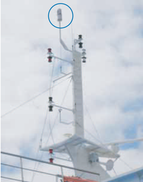
The FLIR M-Series thermal imaging camera is mounted on a pole for a better situational awareness and a better range performance.
