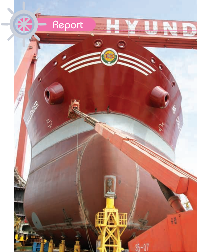
Shipbuilding using the on-ground build method, which HHI successfully completed in 2005 for the first time worldwide
