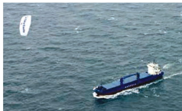
SkySails installation on a cargo ship.
