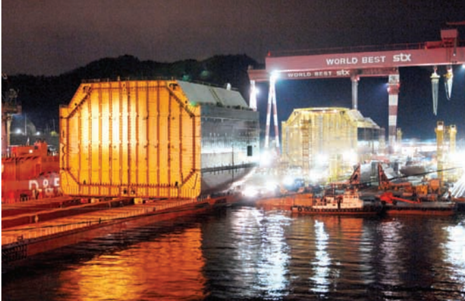
Transportation of a 6,500-ton green block built in land by STXOS, using the semi-submersible heavy-load carrier
