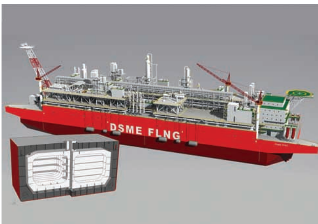
Schematic diagram of the stand-alone type LNG storage cargo hold, developed by DSME, and a LNG-FPSO fitted with that cargo hold
