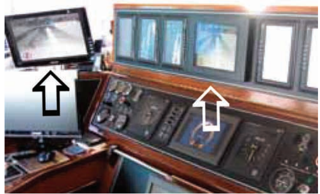
The thermal imaging footage from the FLIR M-Series is continually displayed on one dedicated screen and one multifunctional screen on the bridge of 'El Niño'.
