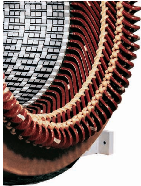
Fig.5 Wound and impregnated stator ready for further assembly
