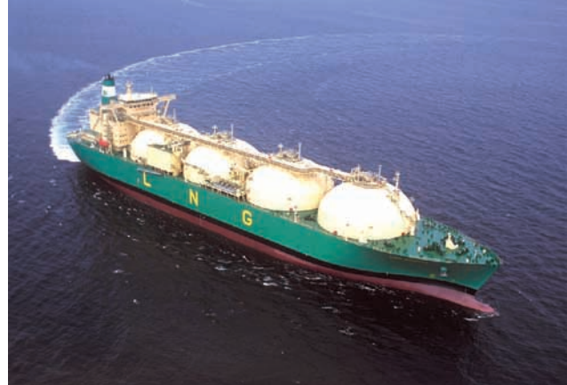
A 137,000m 3 LNG carrier built by HHI
