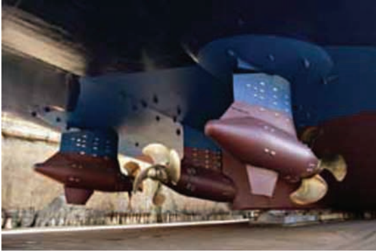
A multi-component Azipod installation (Source: ABB)
