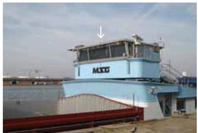
The FLIR M-Series thermal imaging camera is mounted on top of the bridge to provide maximal situational awareness.
