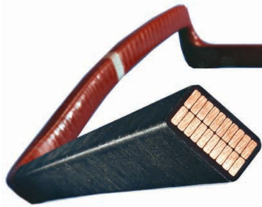
Fig.4 Cross section of an insulated high-voltage coil
