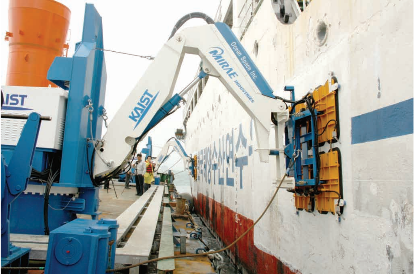
Demonstration of automated ship-to-ship docking
