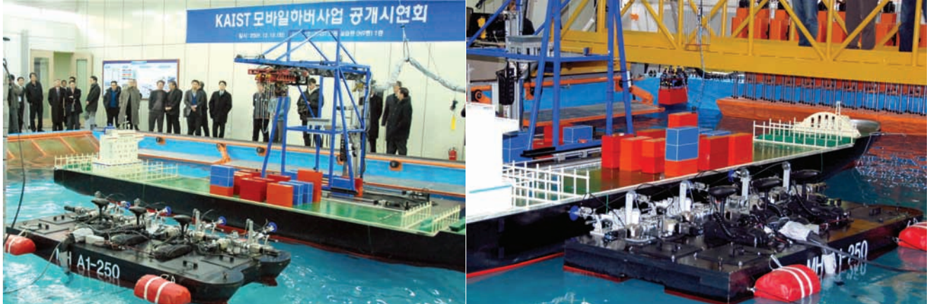
A demonstration of mobile harbor took place on December 15, 2010. The simulation showed the containership being loaded and unloaded with cargoes at the waving sea.
