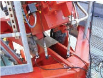
Fig.4 Pressure sensor connected to PXI chassis
