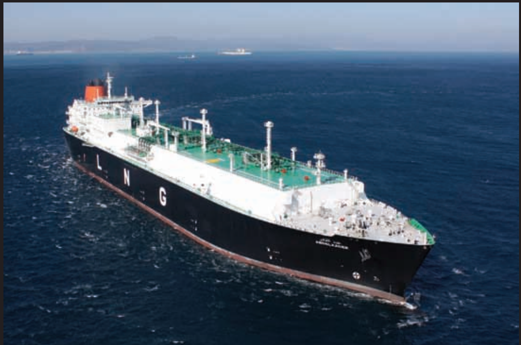
Abdelkader, a 170,000m 3 LNG carrier (HHI, Shipowner: Mol)
