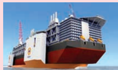
3D model of the 110,000ton semi-submersible heavy transportation vessel (SSHTV)
