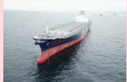
6,500TEU container ship, the world's first vessel built by SSME using the 'on-ground build' method
