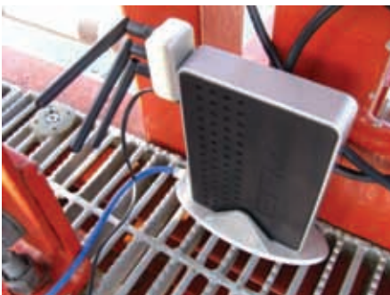
Fig.3 Wireless router installed at the site
