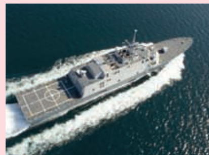
The US Navy's Littoral Combat Ship is powered by Rolls-Royce MT30 gas turbines
