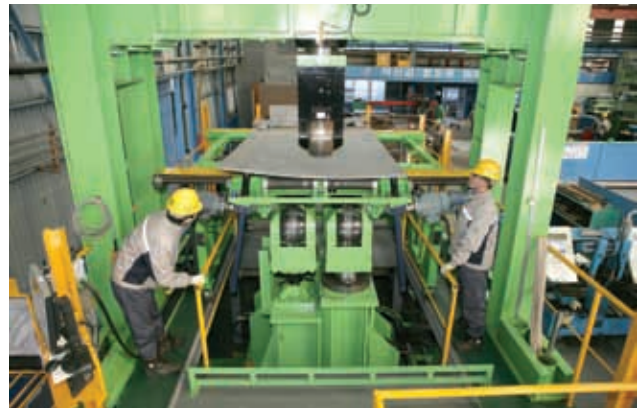
Researchers of the Industrial Technology Research Center of DSME is conducting the test of contour pressing in the Research Center.
