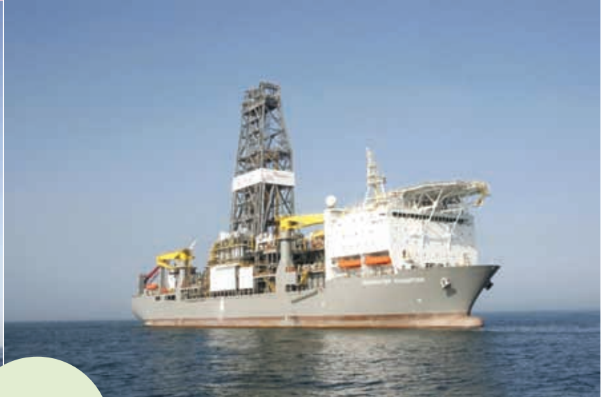
Deepwater Champion, a drillship of HHI which was christened on September 10, 2010. It is a very large drillship capable of drilling as deep as 12km in deepwater regions.
