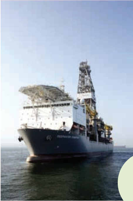
Deepwater Champion, a drillship of HHI which was christened on September 10, 2010. It is a very large drillship capable of drilling as deep as 12km in deepwater regions.
