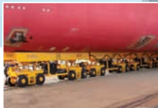
RTP (Transfer System) CAPACITY: 100TON ~ 600TON FOR COMBINATIONS OF UP TO 90,000TON
