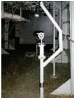
Micropilot M FMR240/ Sounding pipe measurement
