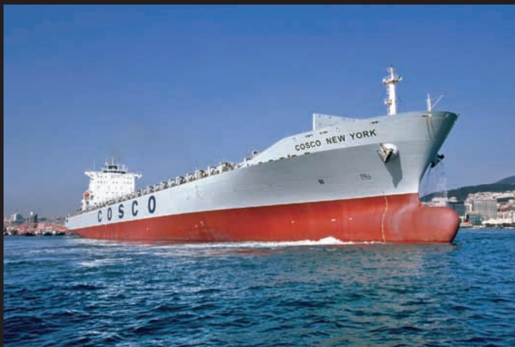
Cosco Newyork 5,100TUE container carriers 294.10 X 32.20 X 21.60 X 12.00 (L X B X D X D, m)
