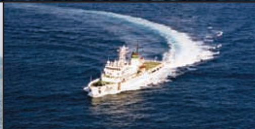
1,500 ton class salvage vessel 98.10 X 14.00 X 6.80 X 4.30 (L X B X D X D, m)
