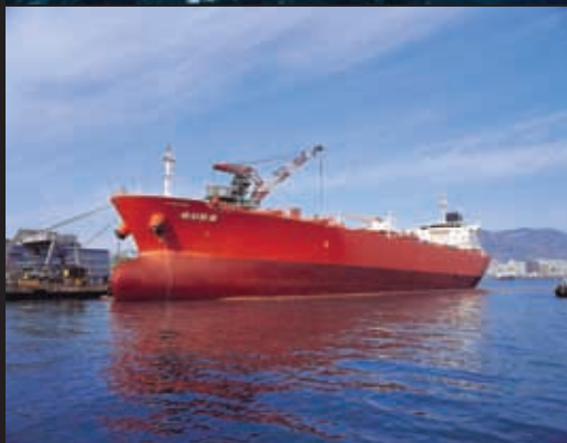
QUDS DWT 45,000 MT chemical tanker 183.20 X 32.20 X 18.90 X 10.97 (L X B X D X D, m)
