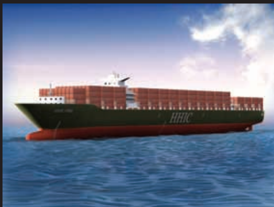
To be named 12,800TUE container carriers 365.60 X 48.40 X 29.80 X 13.00 (L X B X D X D, m)
