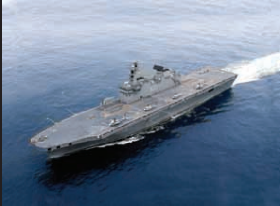
Landing Platform Helicopter (LPH) 199.40 X 31.00 X 20.00 X 6.60 (L X B X D X D, m)
