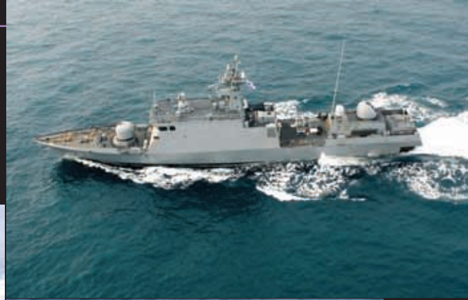
Patrol Killer Guided missile (PKG) 63.00 X 9.10 X 5.00 X 2.50 (L X B X D X D, m)
