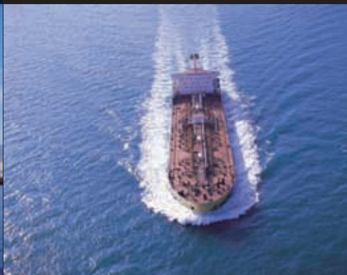
Slot Yosu DWT 37,000 MT chemical tanker 176.80 X 29.60 X 15.15 X 11.56 (L X B X D X D, m)
