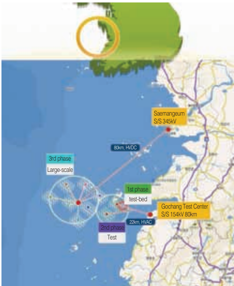
Fig.1 Deployment of offshore wind farm
