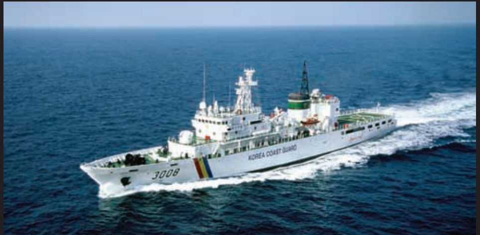
3,000 ton class salvage vessel 110.50 X 15.40 X 7.70 X 4.86 (L X B X D X D, m)
