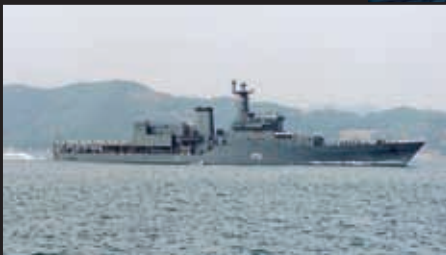
Offshore patrol vessel 101.90 X 11.50 X 6.00 X 3.50 (L X B X D X D, m)
