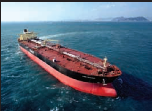
Dubai Princess DWT 114,000 MT crude oil tanker 250.00 X 44.00 X 21.40 X 13.60 (L X B X D X D, m)
