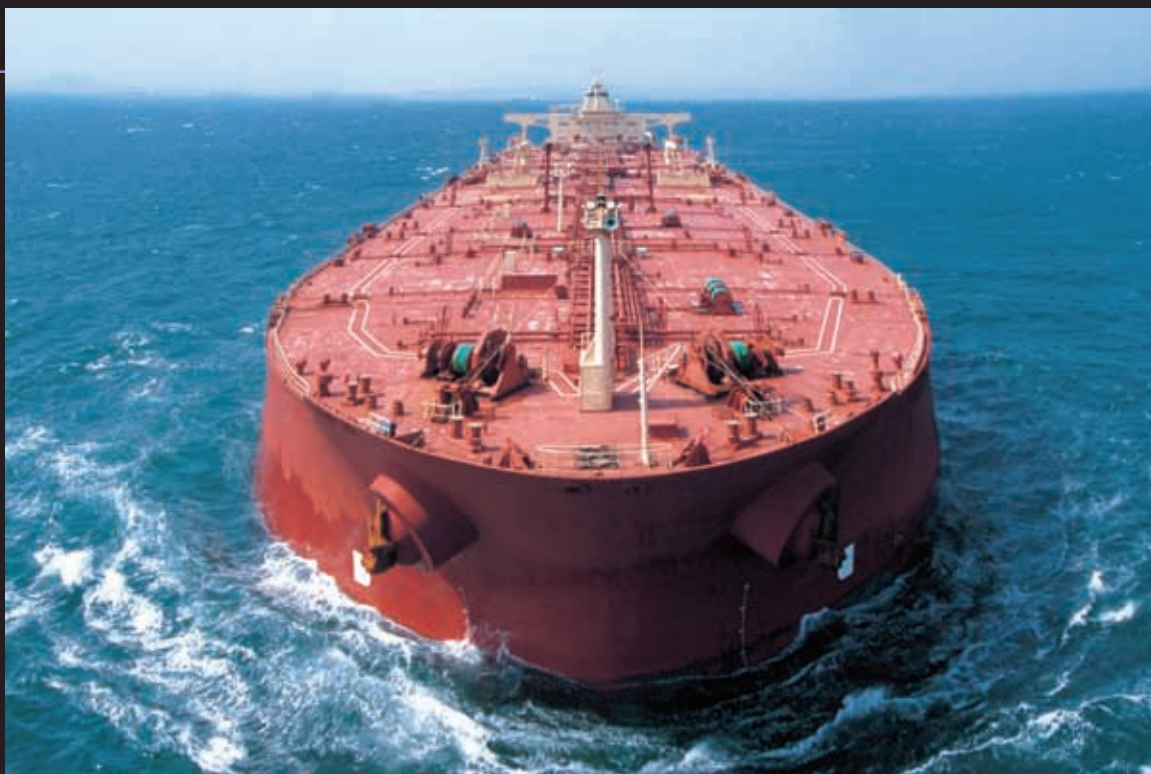
To be named DWT 320,000 MT VLCC 333.00 X 60.00 X 30.50 X 21.00 (L X B X D X D, m)
