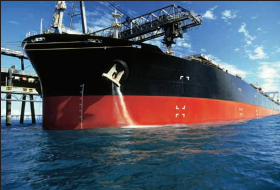
To be named DWT 180,000 MT bulk carrier 292.00 X 45.00 X 24.75 X 16.50 (L X B X D X D, m)
