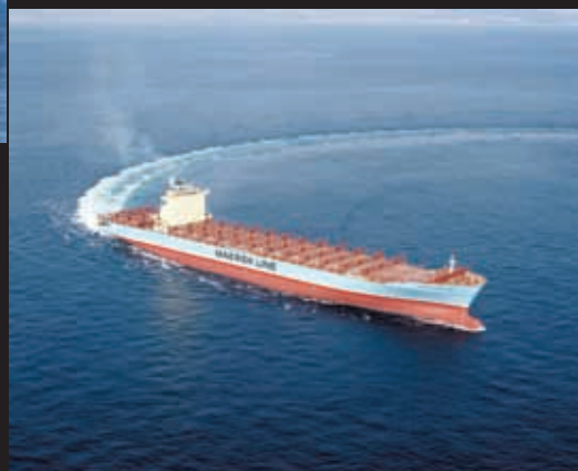
Maersk Kowloon 8,100TUE container carriers 300.00 X 40.00 X 24.60 X 12.00 (L X B X D X D, m)
