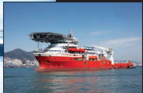
Diving support vessel 115.40 X 22.00 X 9.00 X 7.15 (L X B X D X D, m)
