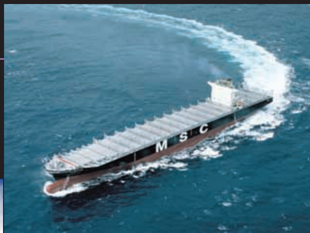
MSC MAEVA 8,100TUE container carriers 325.00 X 42.80 X 24.60 X 13.00 (L X B X D X D, m)
