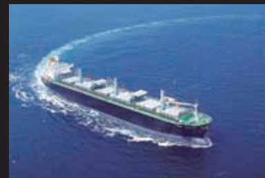
Keoyang Noble DWT 48,000 MT woodchip carrier 222.00 X 32.00 X 22.70 X 10.70 (L X B X D X D, m)
