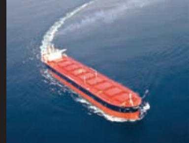
Hanjin Roberts Bank DWT 135,000 MT bulk carrier 267.00 X 43.00 X 23.10 X 16.00 (L X B X D X D, m)
