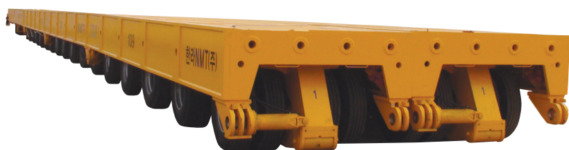
MTP (Module Transporter) CAPACITY : 60ton ~ Over 30,000ton with Multicoupling System
