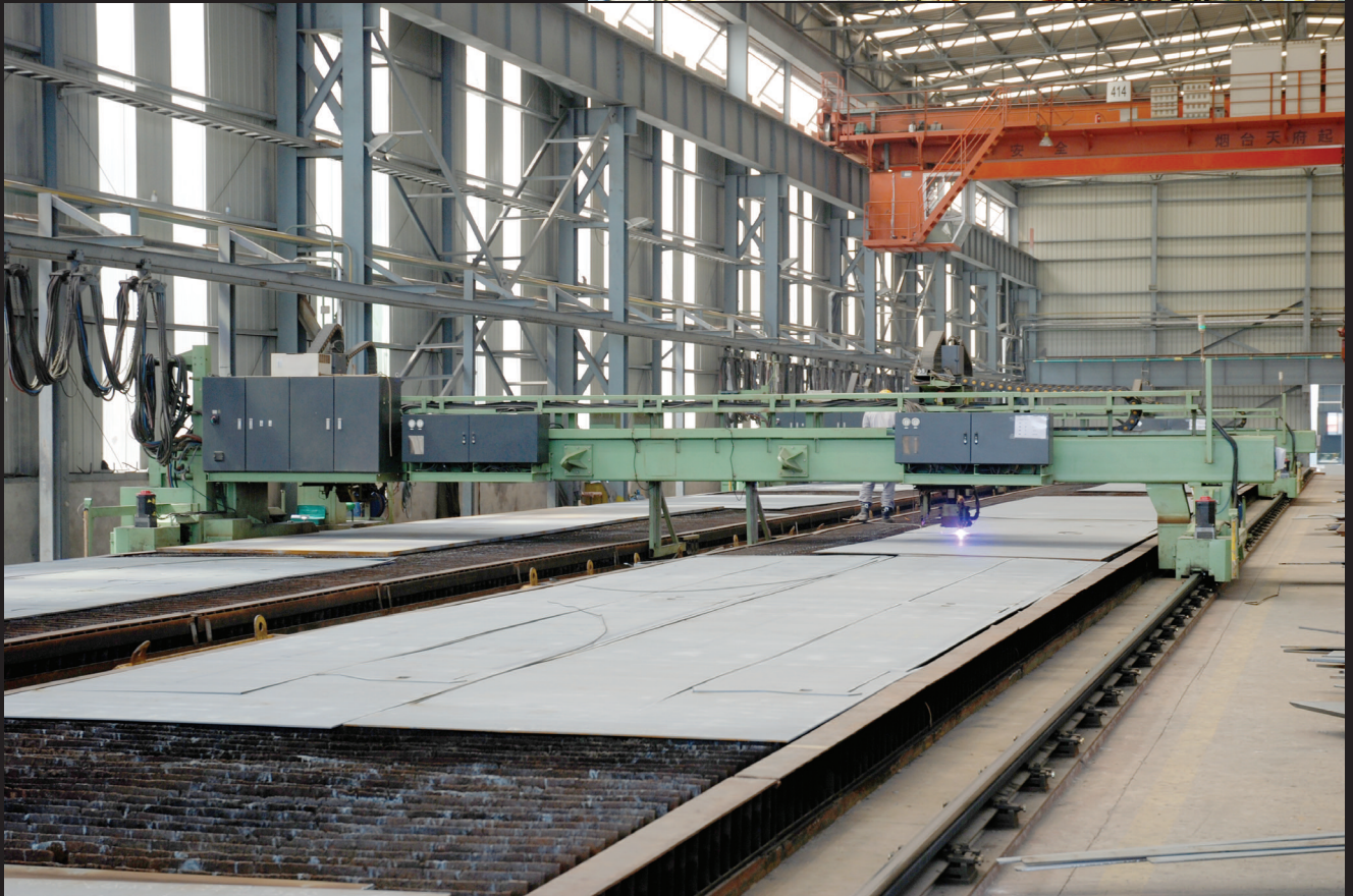
The steel cutting site and steel cutting work in the No. 4 factory
