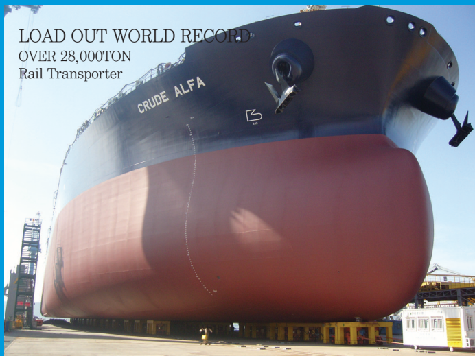
Coupled Module Transporters with Ship Section Carriers
