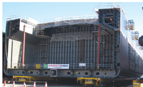
Coupled Module Transporters with Ship Section Carriers
