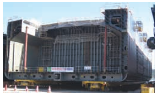
Coupled Module Transporters with Ship Section Carriers
