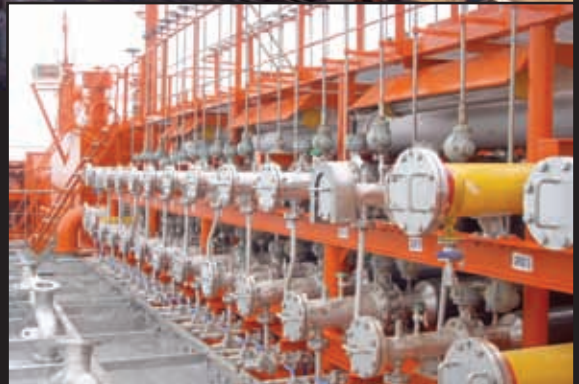
No. H1139~40 11,300DWT stainless steel chemical tanker manifold (ship owner: Crystal Pool Ltd. of Finland)
