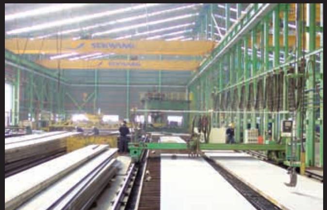
CNC steel cutting machine in the No. 2 factory (No. 2 Yard), a block factory owned by Sekwang Heavy Industries located in Onsan Industrial Complex (currently outsourced)
