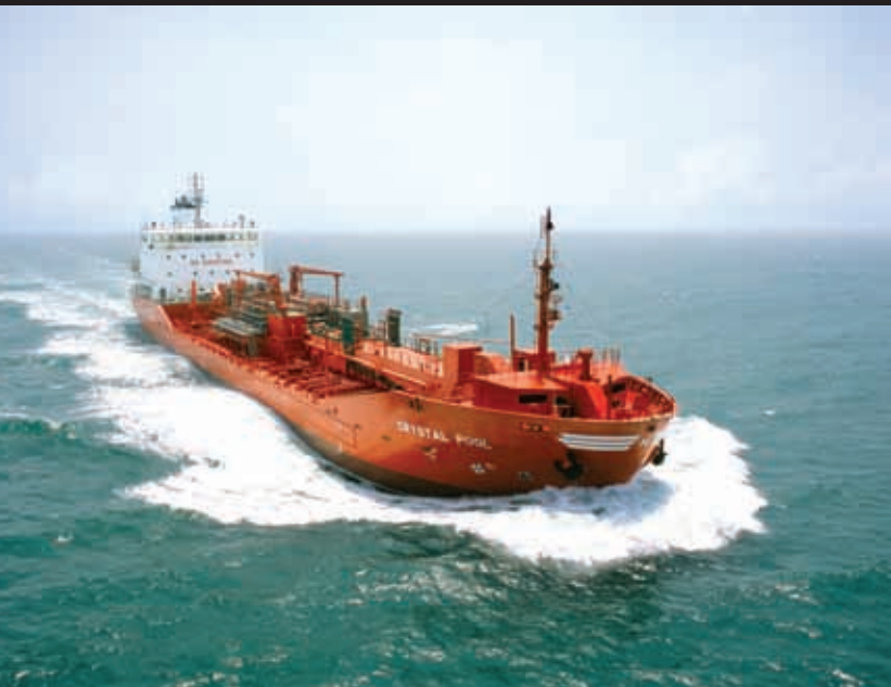
Trial operation of No. H1139~40 11,300DWT stainless steel chemical tanker (ship owner: Crystal Pool Ltd. of Finland)
