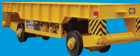
RTP (Rail Transporter) CAPACITY : 100ton ~ Over 30,000ton OPERATING METHOD : AUTO MOBILE
