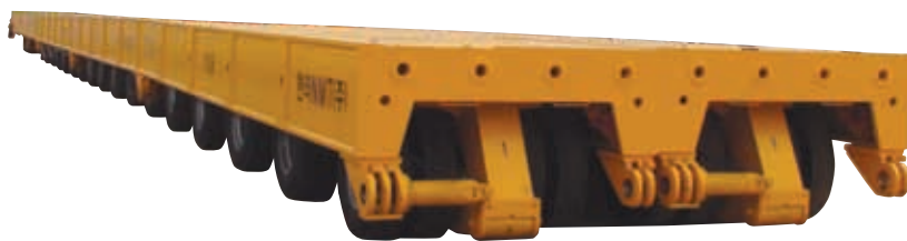
MTP (Module Transporter) CAPACITY : 60ton ~ Over 30,000ton with Multicoupling System
