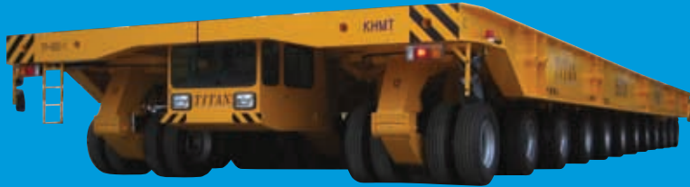
SSC (Ship Section Carrier) CAPACITY : 50ton ~ Over 1,000ton with Multicoupling System
