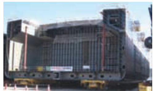
Coupled Module Transporters with Ship Section Carriers
