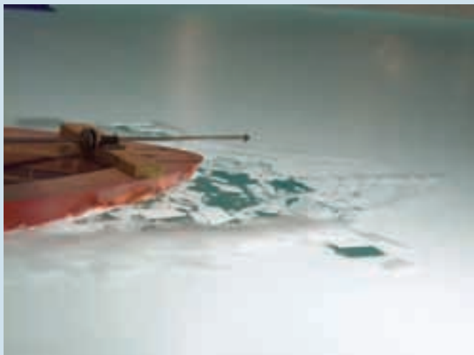
The model ice breaking ship is breaking the ice with its stem and stern in a test.
